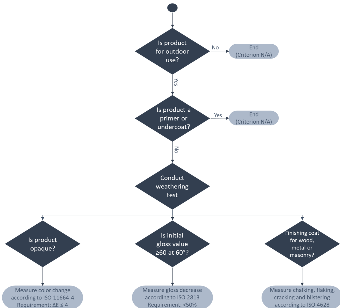
FIGURE 7. LOGIC FOR DETERMINING APPLICABLE REQUIREMENTS IN SUB-CRITERION 2(E).
